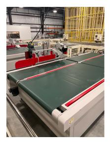
The UM-ATE-2700-HD has United's movable table which eliminates operators from physically pushing mattress from the sewing head. Table returns, as well, to position mattress back into sewing position.
