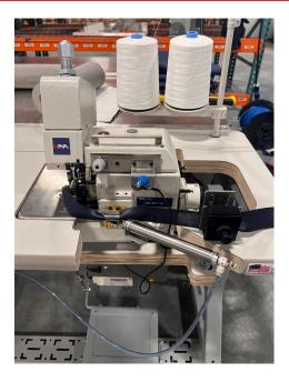
The UM-401-700 half cap bucket maker for the single side beds and high production environment. Joins the thickest border material to the heaviest of panels in one operation.
