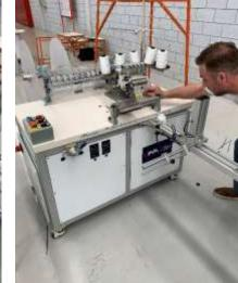
The UM-2400-FAUX automatically sews faux tape seams to borders to simulate pillow top or continental beds with a border and binding tape. This machine is versatile for other tape applications.
